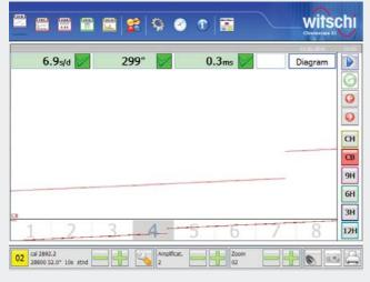
The rate deviation is continuously drawn on the screen. Measured values for rate deviation, amplitude and beat error are displayed numerically.
