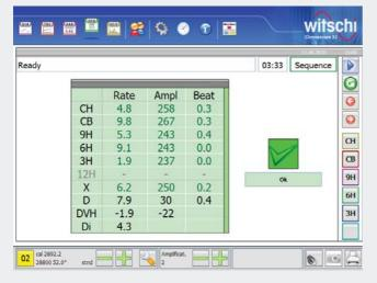
This neatly structured table clearly displays the measurement results in each position as well as the average and the largest difference between all positions and particular ones.
