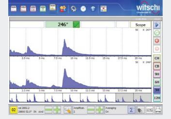
The Scope function graphically displays the acoustic beat noise of the watch. A detailed analysis of the beat noise, i.e. of the state of the escapement, can be carried out. The display can be switched from one to two horizontal axes. Thereby, the averaging of the signals of 1, 10, 20 and 50 beat noises is possible.
